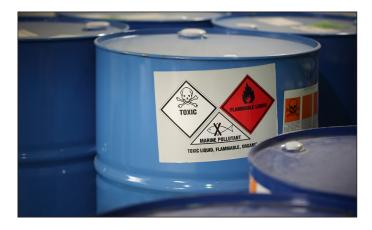
The two primary hazards associated with flammable and combustible liquids are explosion and fire. Safe handling and storage of flammable liquids requires the use of approved equipment and practices per OSHA 29 CFR 1910.106. OSHA will also accept compliance with the most current version of NFPA 30.
